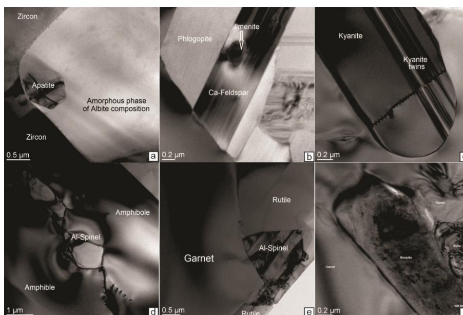
Figure – TEM images of mineral inclusions in Mg-Ca-Fe-garnets from terrigenous deposits of Middle Bug area (Ukrainian Shield).
